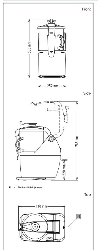
Electric Supply voltage: 200-240 V/1N ph/50/60 Hz Electrical power max.: 1.5 kW **Total Watts:** 1.5 kW Capacity:
